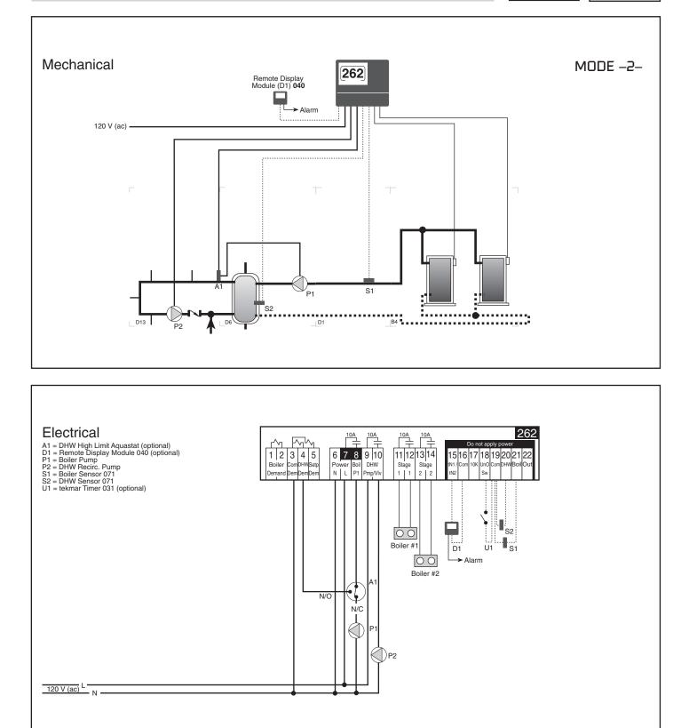
*Note:* This is only a concept drawing. The designer must determine whether this application will work in his system and must ensure compliance with code requirements. Necessary auxiliary equipment, isolation relays (for loads greater than the specified tekmar internal relay ratings), and other safety and limit devices must be added.
